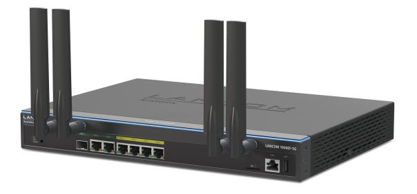
High-performance multi-WAN VPN gateway for SD-WAN with 5G modem, two Gigabit Ethernet WAN ports and fiber-optic SFP port for high-speed networking
