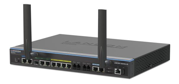
High-end router for SD-WAN scenarios with two VDSL Super Vectoring modems and dual-SIM LTE Advanced backup
